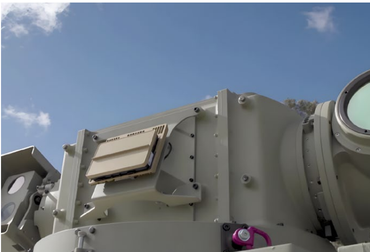
EchoGuard as targeting sensor on EOS Titanis Counter-UAS system.
